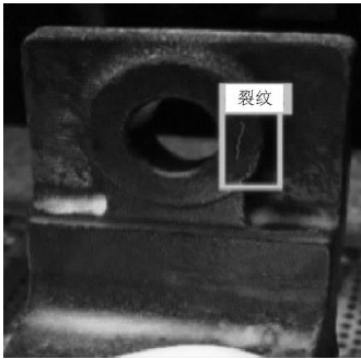
图 5 小缺陷检测效果 Fig.5 Detection effect of small defects
